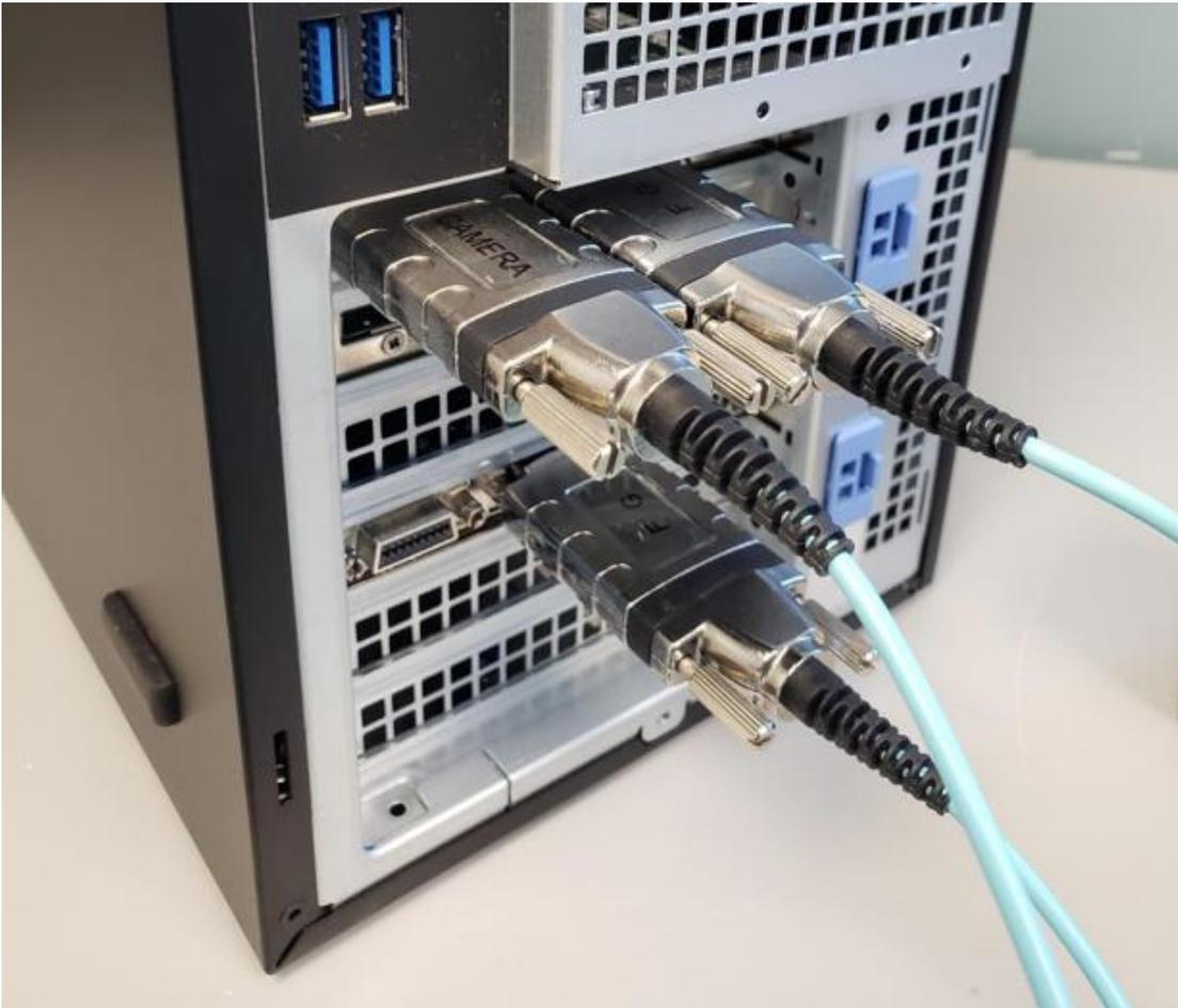
The AOC cable is a directional cable, so make sure to check the terminal mark carefully when connecting. In the *Master connection*, the terminal marked CAMERA must be connected to the camera, and the other terminal marked Frame Grabber (FG) must be connected to the J3 connector (CLHS Input, away from the motherboard) on the Master board.
