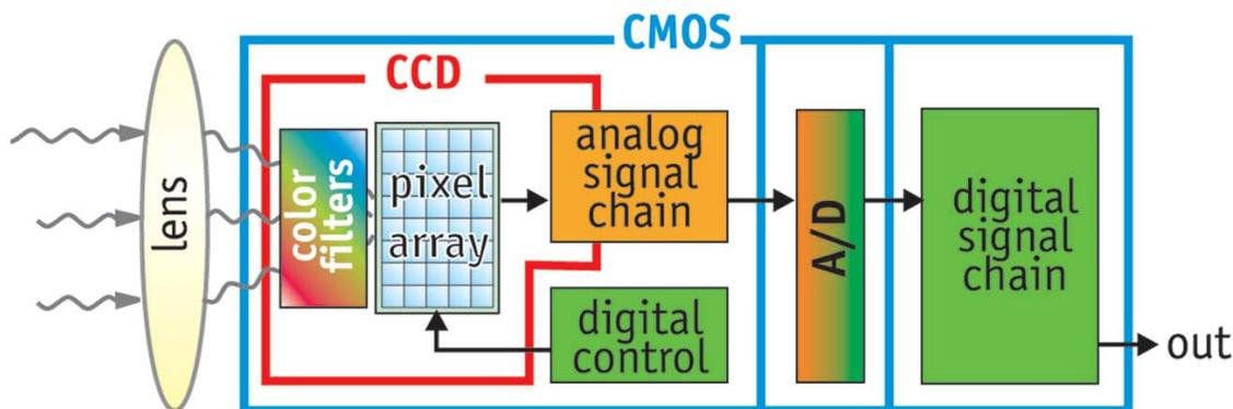
*CMOS imagers can be fabricated with more “camera” functionality on the chip. This offers advantages in size and convenience.*
